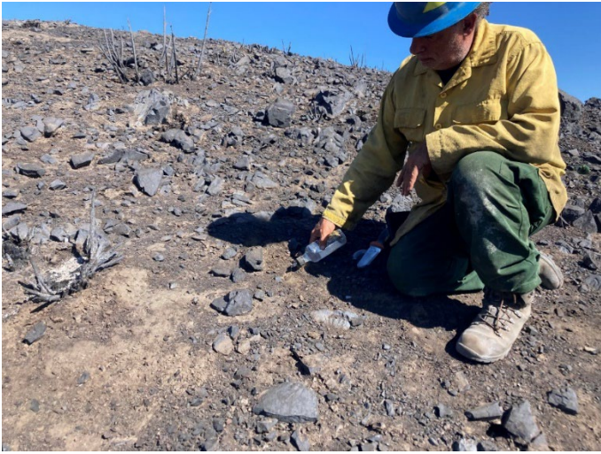
Eric Nicita pours water onto burned soil to test for water repellency
